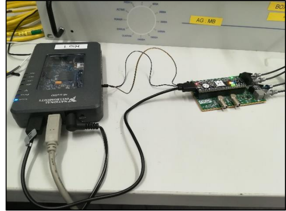
Figure 1- NI myRio connected to ADC Dongle
